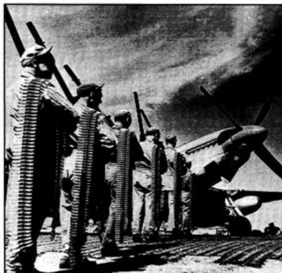
Armourers each carrying one 0.50 calibre machine gun and a belt of ammo prepare a P-51 Mustang for an escort mission.
