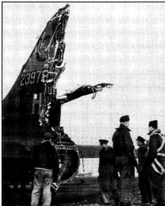
"Thru Hel'en Hi water" returned to base after a direct hit on the tail. The tail gunner was uninjured, fortunate that he was checking the tail wheel when the shell hit. Time and time again the B-17 proved it could sustain major damage and keep on flying.
