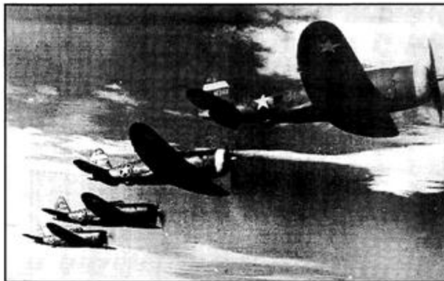
A flight of P-47 Thunderbolts. Each aircraft packed a formidable eight high muzzle velocity 0.50 calibre machine guns.
