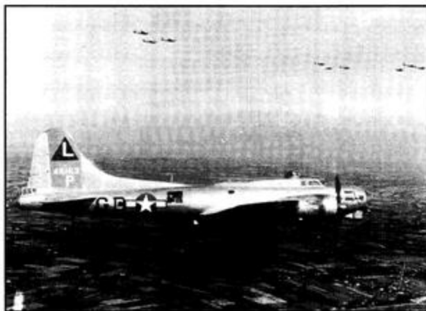
The B-17G Flying Fortress without camouflage paint. It was decided to leave the aircraft in its original metal finish in later models because, at the height it flew, camouflage would make little difference. In fact, without the paint it was a lighter and faster aircraft.
