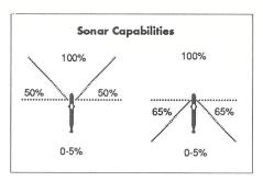
Figure 5.6: Increased Sonar Capabilities With Towed Array
