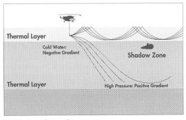
Figure 6.1: Thermal Layers
