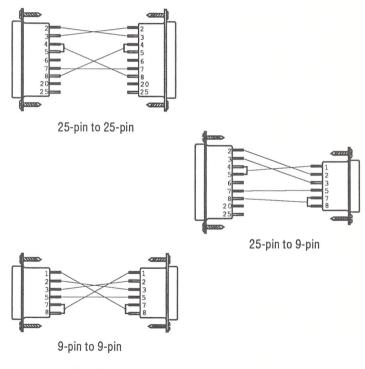
Figure A: Null-Modem Connections
