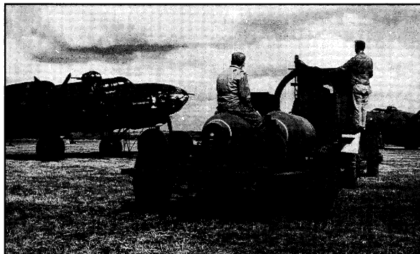
Bomb service truck and trailer approach a flight of B-17F's with 2 one-ton bombs. Exploding fragments from these bombs could travel over a mile in distance.
