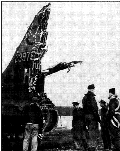
"Thru Hel'en Hi water" returned to base after a direct hit on the tail. The tail gunner was uninjured, fortunate that he was checking the tail wheel when the shell hit. Time and time again the B-17 proved it could sustain major damage and keep on flying.
