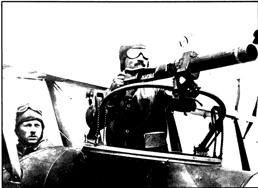
A French aviator uses a specially designed camera to practice lining up a target in the sights of a machine gun.
